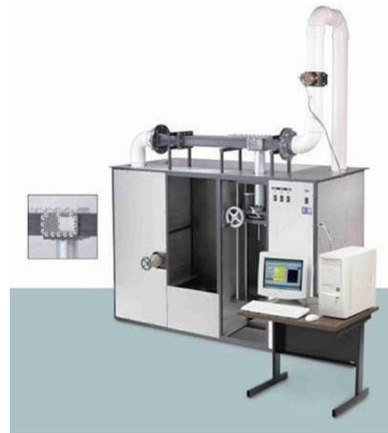
SRICOS-EFA (Scour Rate In COhesive Soil – Erosion Function Apparatus)
