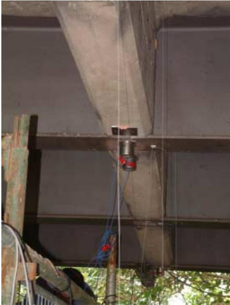
Figure 2.2. Redbank Creek Bridge - showing accelerometers attached to steel girder and concrete diaphragm
