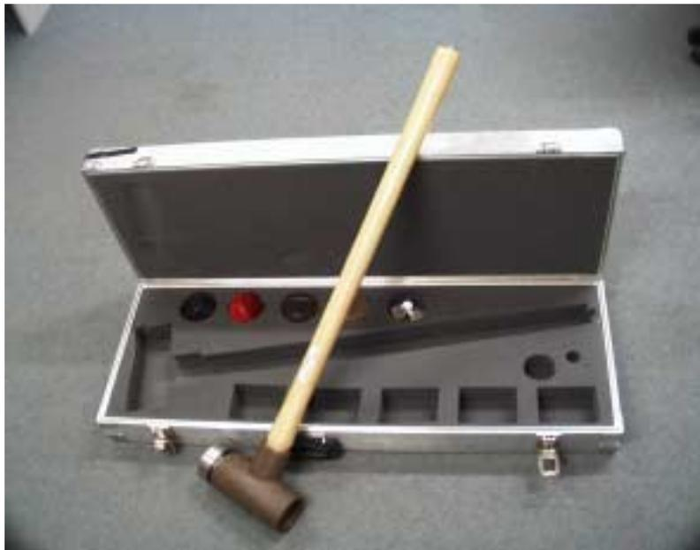
Figure 2.3 The 12 lb Modally Tuned ICP Sledge Hammer used for bridge tests
