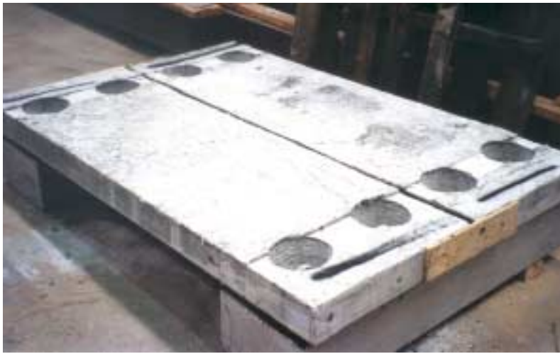
Fig. 12 : Slabs prior to casting of slab to slab joint and slab to beam connections
