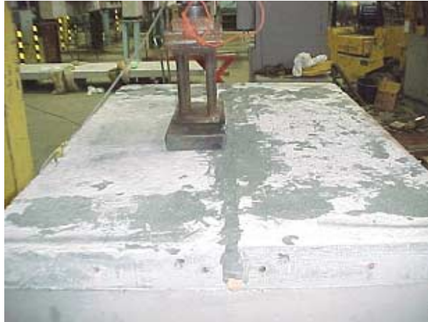
Fig. 14: Prototype slab to slab joint with simulated wheel load adjacent to joint
