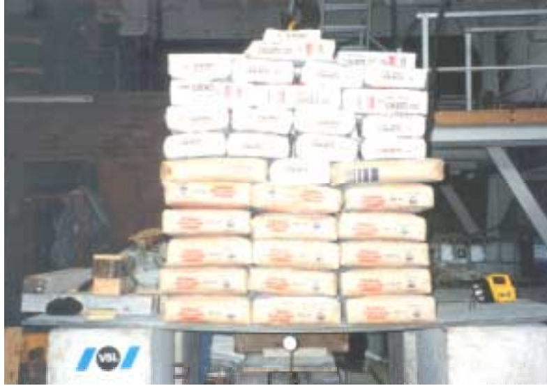
Fig. 8: 25mm thick permanent formwork slab, span 1.3m load 18 kPa
