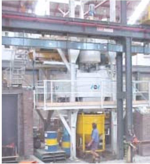
Fig. 5: Mixer for Ductal
