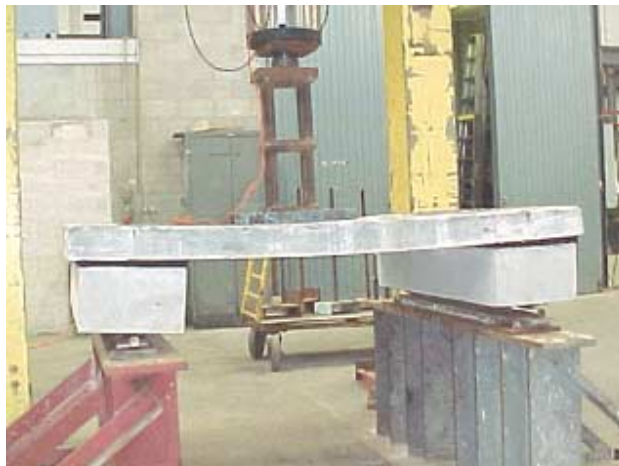
Fig. 15 : Test slab at a simulated wheel load of 250kN
