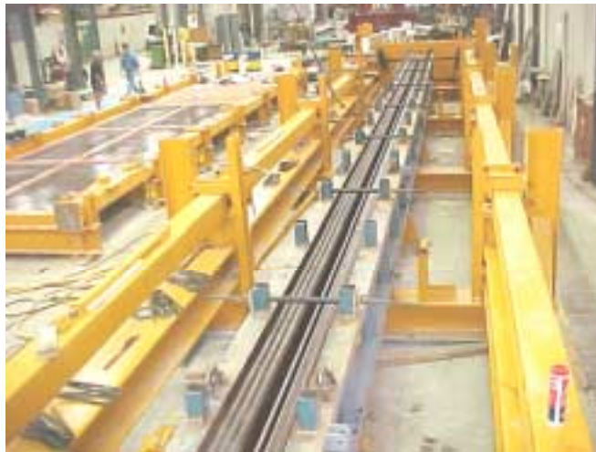
Fig. 6: Forms and pretensioning frame
