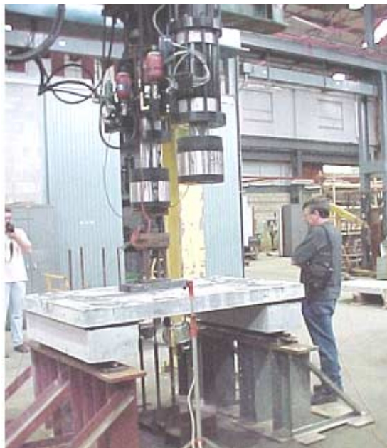
Fig. 13: Test loading of slab to slab joint
