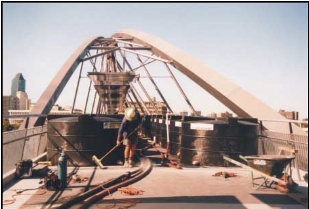
Figure 11: Load testing of main span via water tanks
