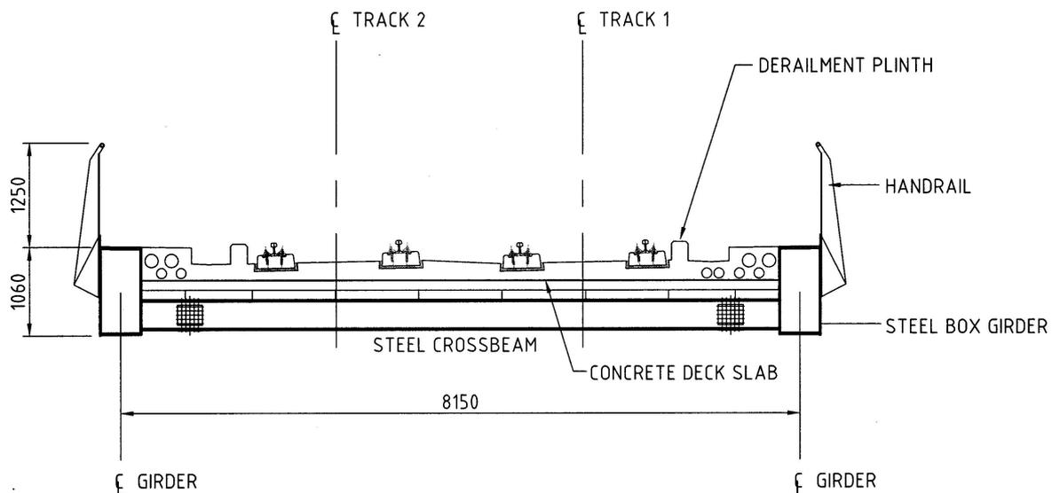
**Figure 2 : Cross Section of Typical Bridge**
