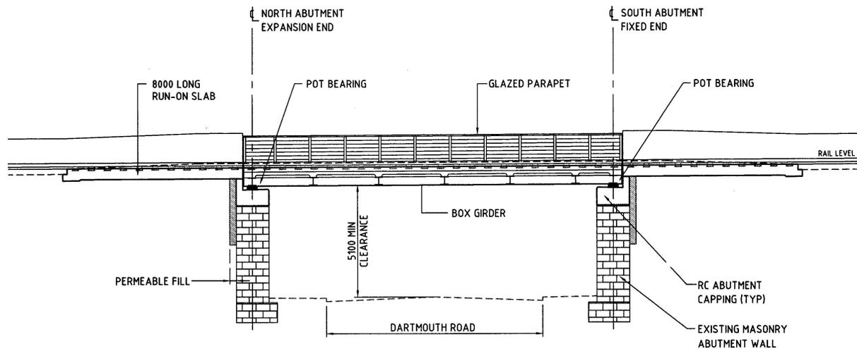
**Figure 3 : Elevation on Typical Bridge**
