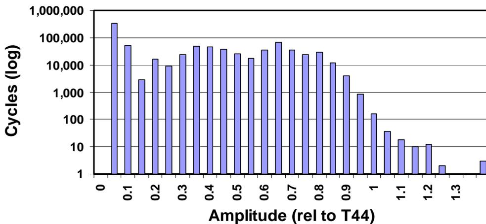
Figure 4: Count of Cycles Versus Amplitude of Response by Rainflow Method
