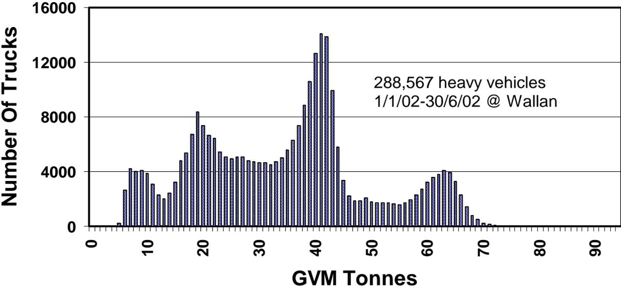
*Figure 2: Histogram of Gross Vehicle Mass, Hume Freeway*
