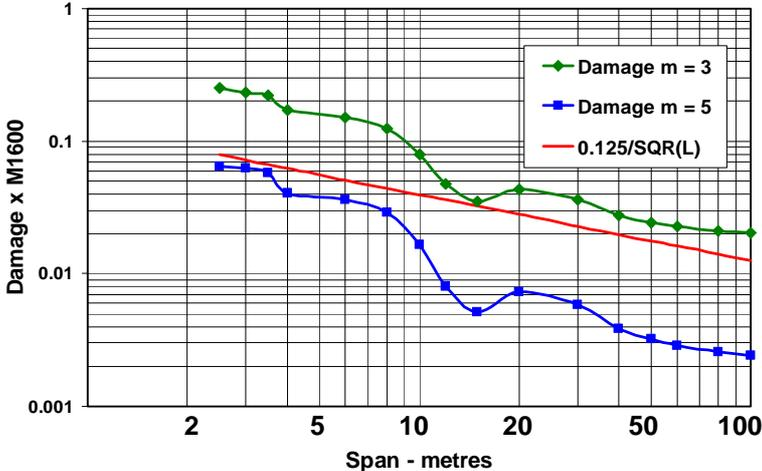
Figure 5: Fatigue Damage per Truck, Hume Freeway, 2001, Versus Span
