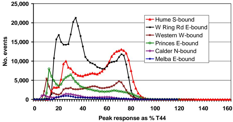
Figure 6: Comparison of Peak Response for Various Routes, Jan-Jun 2001, Span 8.5m
