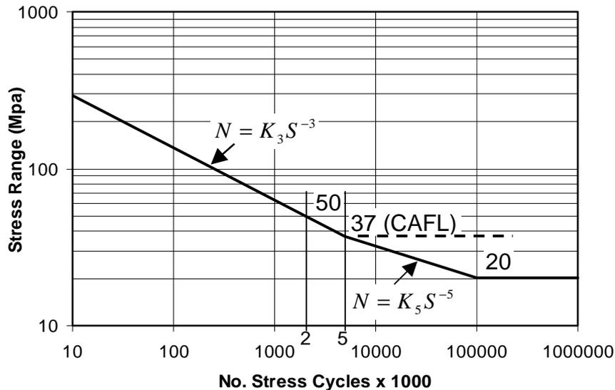
**Figure 1: Design S-N Curve for Detail Category 50 under Variable Amplitude Loading ( $S = 50$  MPa at 2 million, 37 MPa at 5 million and 20 MPa at 100 million cycles)**
