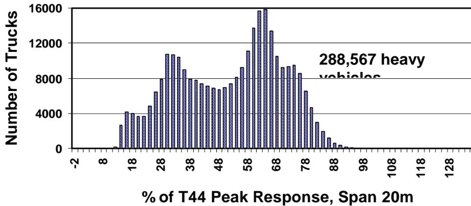
Figure 3: Peak Bending Moment Compared with T44 truck (highest 135%)
