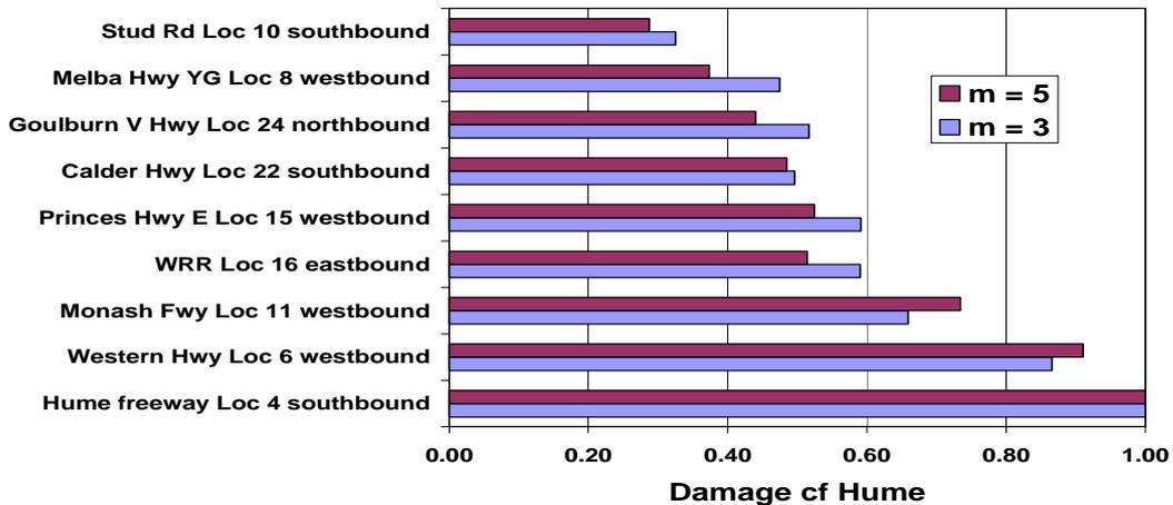
Figure 7: Relative fatigue damage/truck on different routes, compared with Hume Fwy
