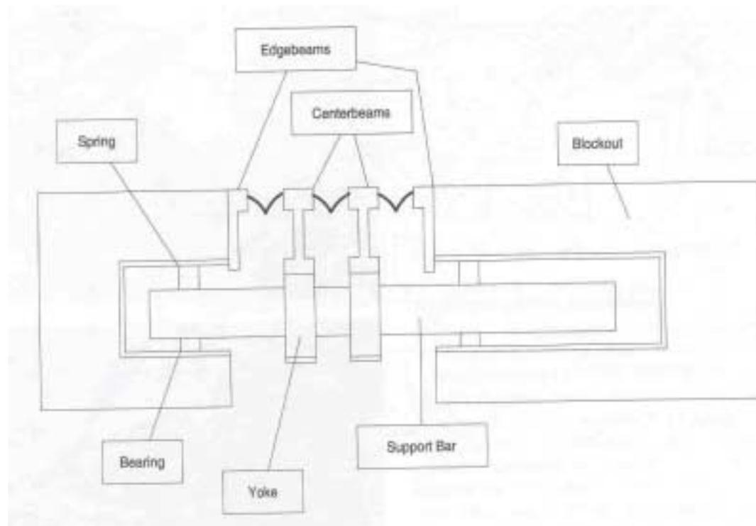
**Figure 1: Typical Single Support Bar Design MBEJ**
