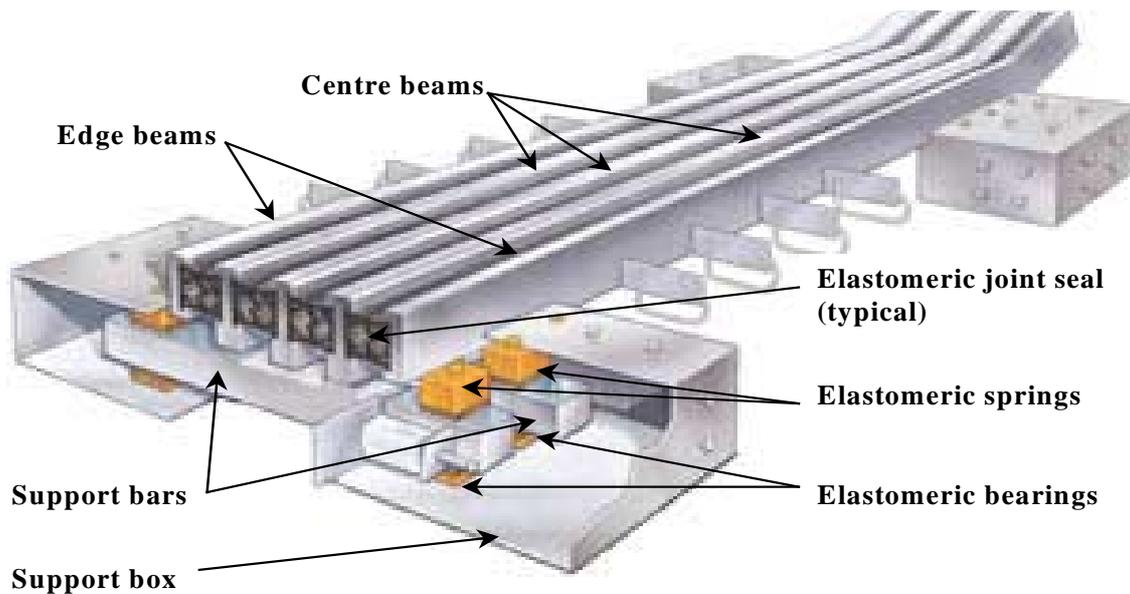
**Figure 2: Typical Multiple Support Bar Design MBEJ**
