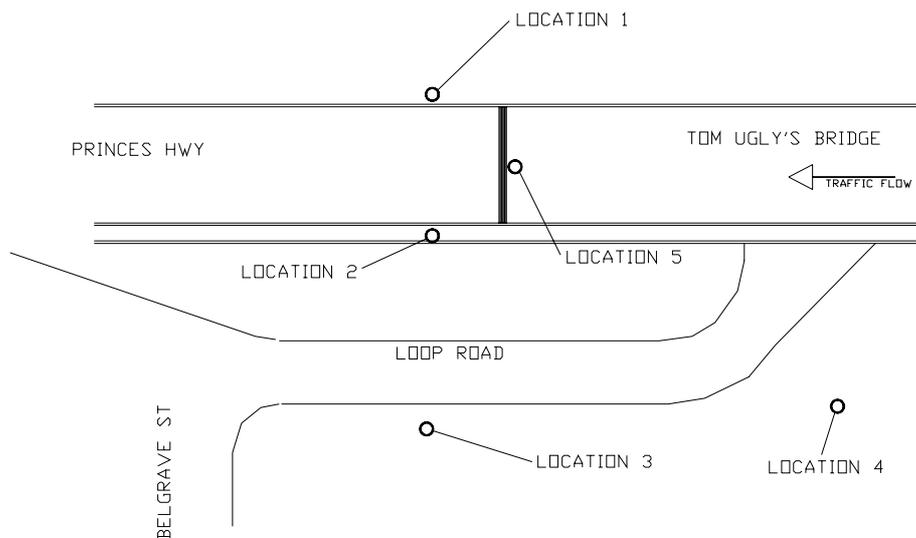
*Figure 8: Site Plan Showing Noise Measurement Locations*
