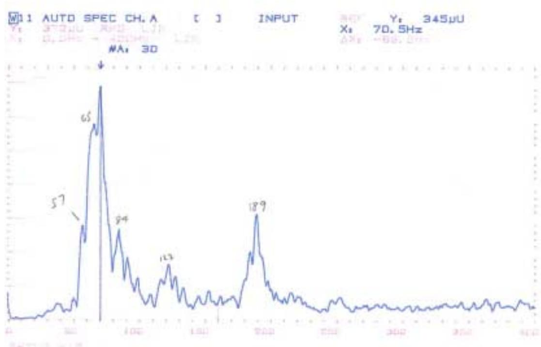
**Figure 5: Transverse Beam Vibration Spectrum – Anzac Bridge**
