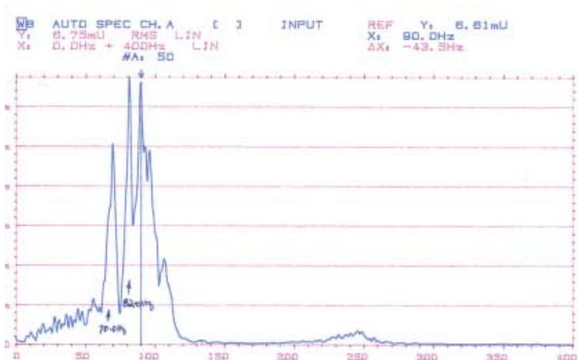
*Figure 3: Transverse Beam Vibration Spectrum – Tom Ugly's Bridge*
