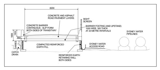
Figure 1: Cross Section at Footing, Liverpool Parramatta Bus Transitway
