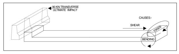
Figure 5: Diagrammatic Isolated Footing Loads for Impact Barrier
