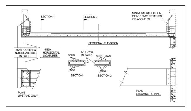
Figure 6: Footing Reinforcing Liverpool Parramatta Bus Transitway
