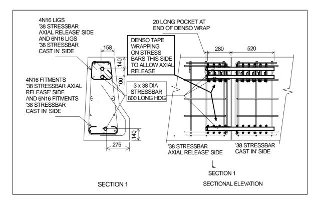
Figure 7: Barrier Expansion Joint - Liverpool Parramatta Bus Transitway
