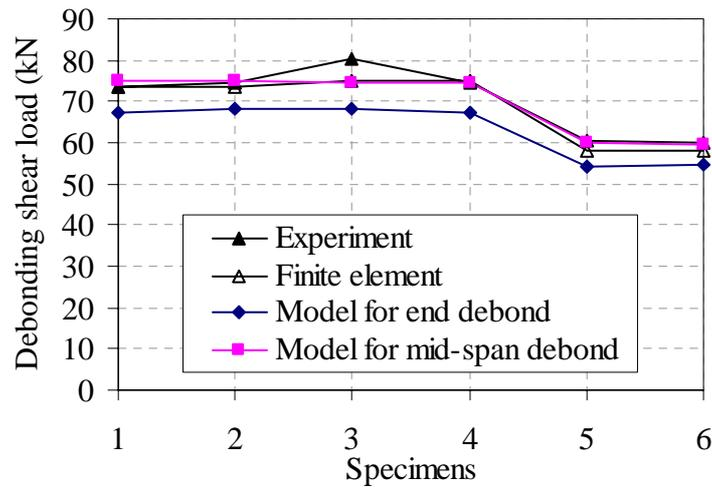
**Figure 6: Comparison between the theoretical models and experimental results**
