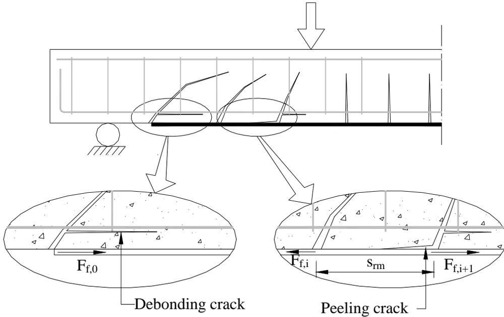
**Figure 5: Failure mechanisms**
