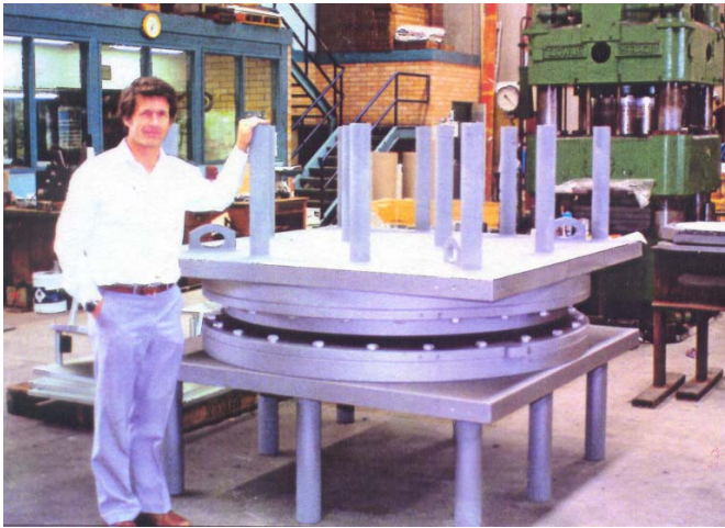
Fig 12a. Anzac Bridge, Sydney, and the largest pot bearing in Australia (with a capacity of 46000kN SLS), designed and tested to 50000kN by G. Davidson whilst at Hercules Engineering, 1992.
