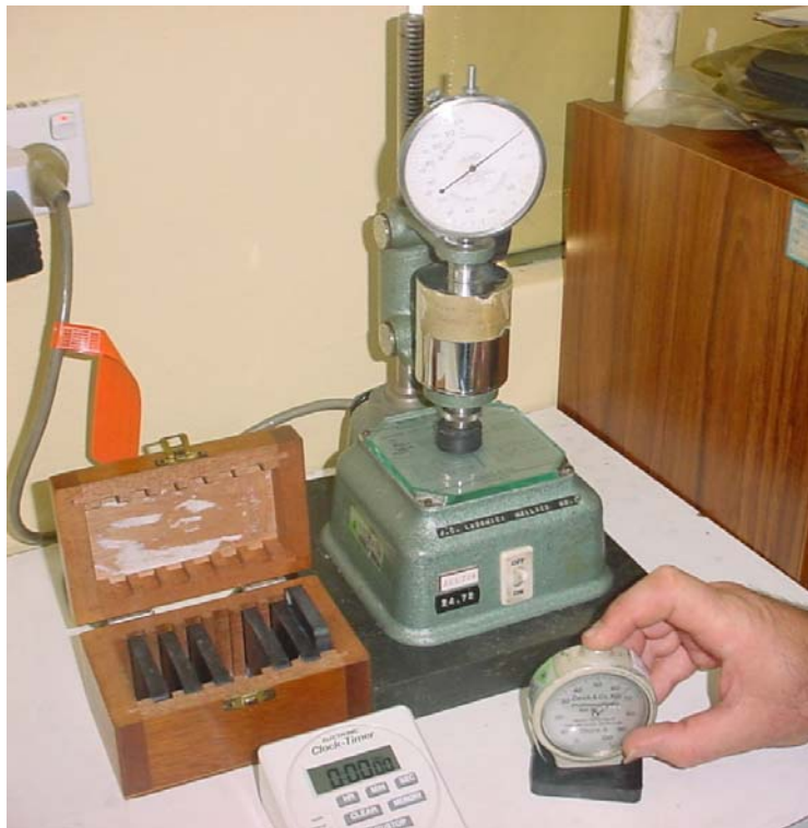
Fig 8a. IRHD Hardness Tester (International Rubber Hardness Degrees) in the background. This is a laboratory machine operated at controlled temperature (23 +/- 2degC), and carefully timed at 30 seconds (method N as specified).
