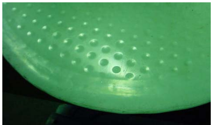
Fig 2b. There are two principal ways that PTFE can experience the distress shown at right, namely
