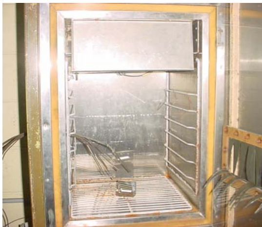
Fig 11b. Left Top – Tension and compression set samples undergoing accelerated aging at 70°C.
