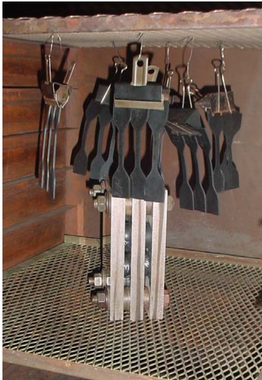
Fig 11a. Top- Samples for testing are moulded and cut from thin sheets. This shows some of the knives and samples for the tension test, the quad shear test, the tear test, compression set and hardness buttons. Most are quarterly tests, although hardness checks are required on EVERY batch, and quad shear is yearly (with low temperature and ozone tests).
