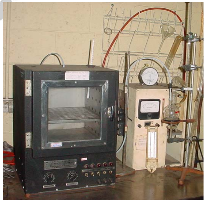
Fig 11b. Left Top – Tension and compression set samples undergoing accelerated aging at 70°C.
