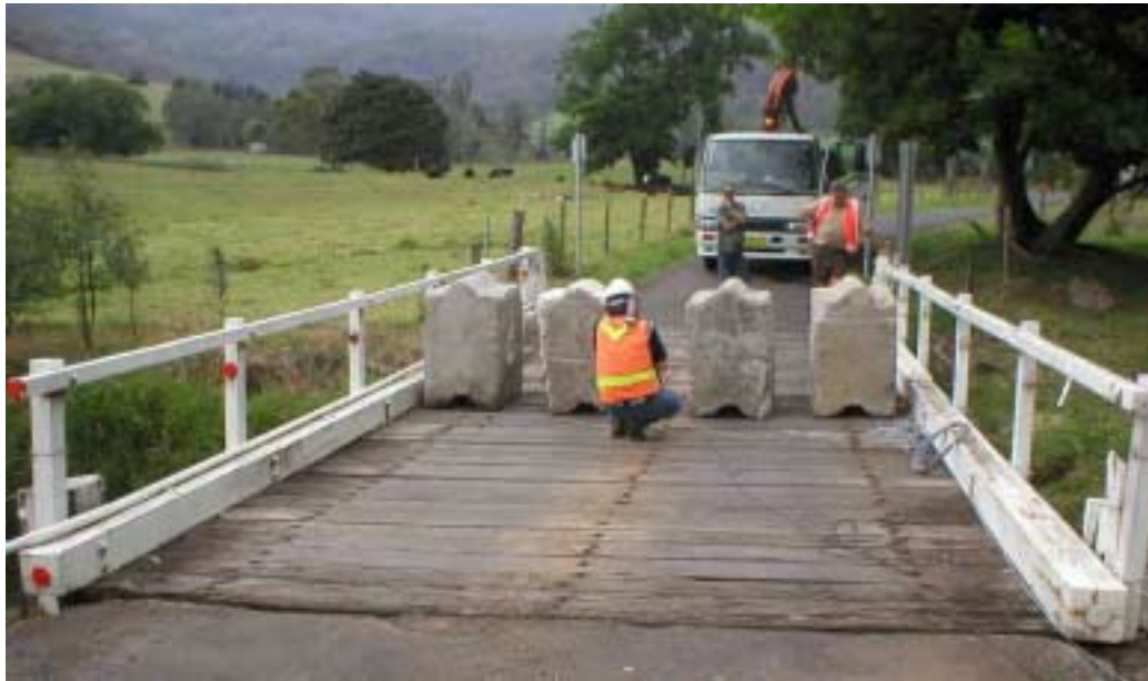
Figure 6: Testing with mass applied at mid span
